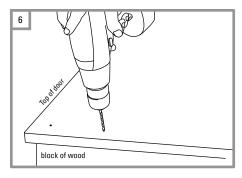
Once the handing has been chosen, remove the door using the quick release hinges. Place door on to a clean and smooth scrap piece of wood and carefully drill out the selected holes for the handle bolts.
