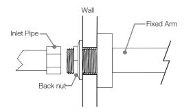
1. Secure arm in place using the back nut provided (See diagram above)
