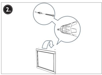
Drill two holes in the marked positions using an 8mm drill bit to a depth of 55mm. Insert the wall plug supplied in the ficing screw, leaving sufficient head showing to slide into the mirror wall brackets.
