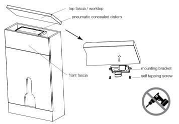
The unit can be mounted behind the front fascia or under the worktop of a WC furniture unit. Make a suitable pilot hole and use the self tapping screws supplied if mounting onto a wooden fascia.
