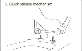
This toilet seat is designed for quick and easy removal when cleaning the toilet pan. To quickly release the seat, lift the lid and seat up to a vertical position. From there, lift one side of the seat up to disengage the pin followed by the opposite side. the seat should easily lift away from the pins. To replace the seat align the sockets with the pins and firmly press down until the seat is engaged into position.
