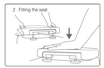
Align and insert the hinge anchors into the hinges on the seat and firmly press down until the seat is engaged into position. Adjust the hinge anchors to make sure the seat lines up with the edges of the toilet pan. When you are satisfied the seat is in the correct position, remove the seat from the hinge anchors (see step 3) and fully tighten the screw (shown in step 1). Place the cover plates over the hinge anchors. Replace the seat and 'push' into position.
