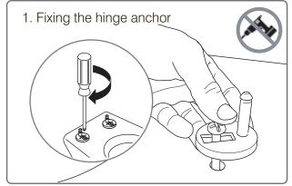
Place the Top Fix Inserts into the fixing holes in the toilet pan. Insert the screws into the Hinge Anchors using the washers provided between the pan and anchor. Begin to tighten the screws until they are loosely secured, to allow for adjustment of the seat on the pan. Do not fully tighten at this stage.
