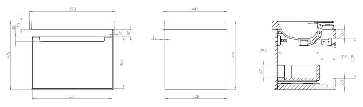
Diagrams not to scale All dimensions in mm Tolerance of +/-5mm
