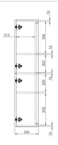
Diagrams not to scale All dimensions in mm Tolerance of +/-5mm
