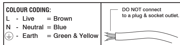
WIRING DIAGRAM - MAINS SUPPLY
