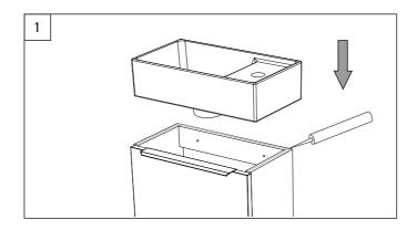
Once the basin is plumbed in, finish by securing it to the furniture unit along the top face of the side panel with silicone sealant (not supplied).
