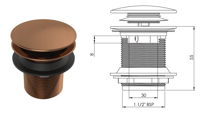
DIAGRAMS NOT TO SCALE | ALL DIMENSIONS IN MM TOLERANCE OF  $\pm$  5MM
