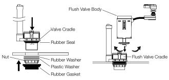
Ensure that the Flush Valve is assembled and fully tightened as shown.
