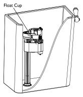
The fill valve is supplied set at a height suitable for the cistern tank. Please ensure that all connections are fully tightened before progressing.
