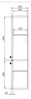
Diagrams not to scale All dimensions in mm Tolerance of +/-5mm
