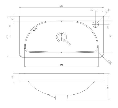
Diagrams not to scale All dimensions in mm Tolerance of +/-5mm
