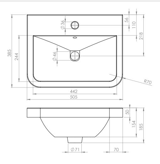
Diagrams not to scale All dimensions in mm tolerance of +/-5mm
