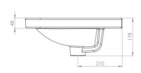
Diagrams not to scale All dimensions in mm Tolerance of +/-5mm
