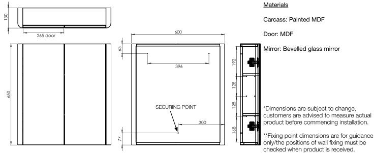
Diagrams not to scale. All dimensions in mm (tolerance of +/-5mm)
