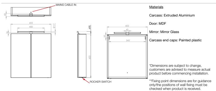
Diagrams not to scale. All dimensions in mm (tolerance of +/-5mm)
