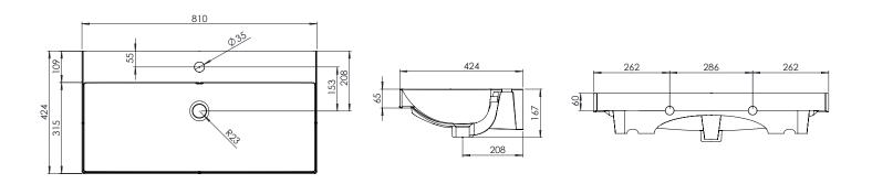
Diagrams not to scale All dimensions in mm Tolerance of +/-5mm
