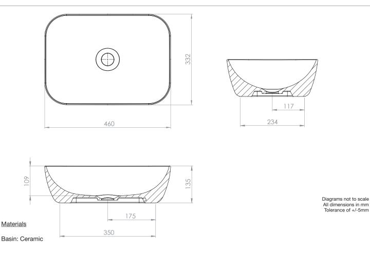
\*\*Dimensions are subject to change, customers are advised to measure actual product before commencing installation. \*\*\* BASIN HAS NO OVERFLOW SO MUST BE USED WITH AN OPEN WASTE
