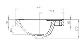
Diagrams not to scale All dimensions in mm Tolerance of +/-6mm
