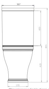
DIAGRAMS NOT TO SCALE | ALL DIMENSIONS IN MM TOLERANCE OF  $\pm$  5MM  $\,$  ALL PRODUCTS CONFORM TO BRITISH STANDARDS
