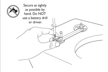
A Remeasure the distance, making sure the 412mm dimension is met and remove the template and add the cover cap.
