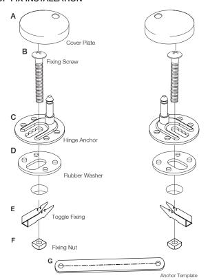
Place the template over the anchor pins, selecting the appropriate hole numbers (on the anchors) so that the 412mm dimension from the front of the pan to the centre line of the template is met.
