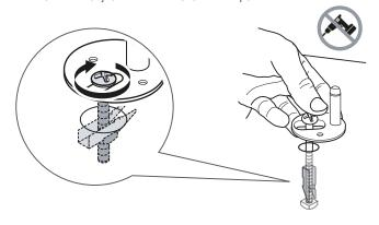
3 Once the 412mm dimension shown above is met and the template is parallel to the back edge, insert the bolts then fully tighten using a screw driver.
