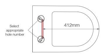
Insert the screws, toggle fixing and nut into the seat fixing holes of the toilet pan as shown using the selected fixing hole of the anchor. Lift the hinge anchor back up to engage the toggle fixing on the underside of the pan. Begin to tighten the screws until they are loosely secured, to allow for adjustment of the seat on the pan.
