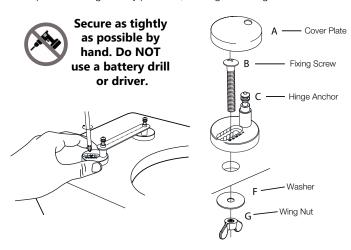
3 Remeasure the distance, making sure the 445mm dimension is met and remove the template and add the cover cap.
