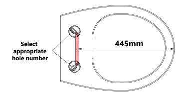
2 Once the 445mm dimension shown above is met and the template is parallel to the back edge, insert the bolts and tighten the underfix components using the key provided, then tighten using a screw driver.
