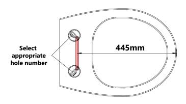
3 Once the 445mm dimension shown above is met and the template is parallel to the back edge, insert the bolts then tighten using a screw driver.
