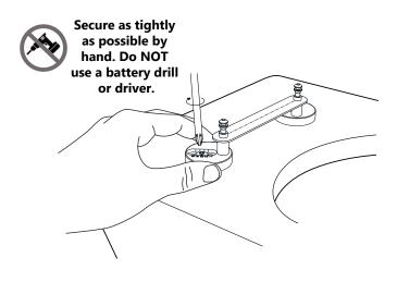
A Remeasure the distance, making sure the 445mm dimension is met and remove the template and add the cover cap.
