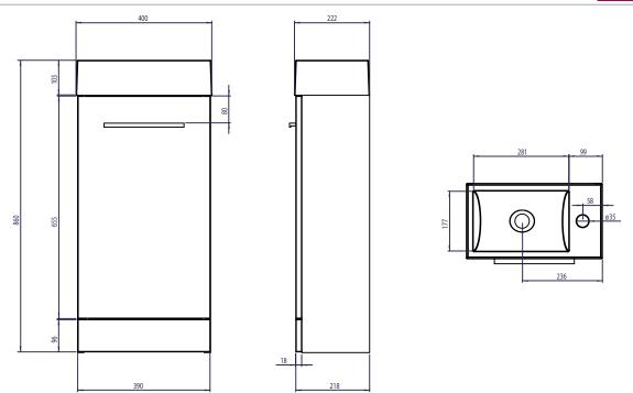
Diagrams not to scale All dimensions in mm Tolerance of +/-5mm
