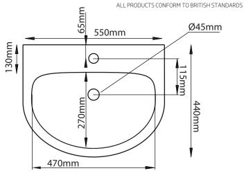
${}^\star \text{Dimensions are subject to change, customers are advised to measure actual product before commencing installation.}$ \*\*Fixing point dimensions are for guidance only. The positions of fixings must be checked when product is received.
