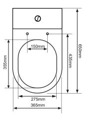
DIAGRAMS NOT TO SCALE | ALL DIMENSIONS IN MM TOLERANCE OF  $\pm$  5MM
