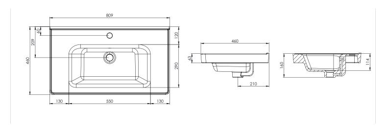
Diagrams not to scale All dimensions in mm Tolerance of +/-5mm
