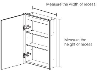
1.2 - Mark out the recess on the wall. Special attention must be taken to ensure there is nothing within the desired recessed space.
