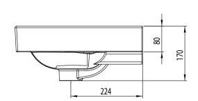
Diagrams not to scale All dimensins in mm tolerance of +5mm
