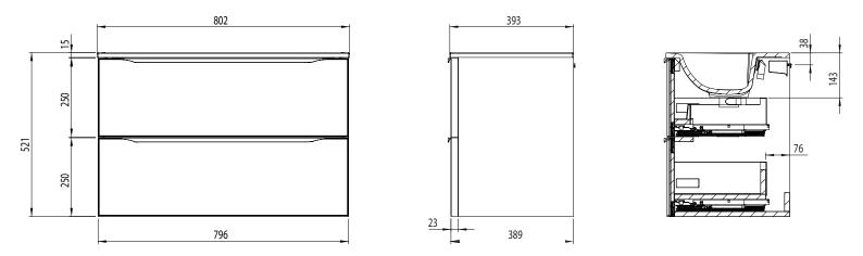
Diagrams not to scale All dimensins in mm tolerance of +5mm
