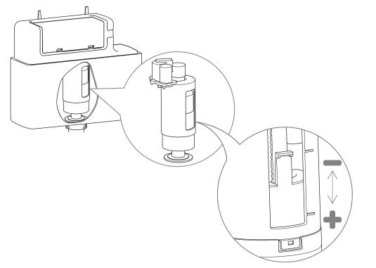
By adjusting the flush valve the flushing volume can be altered
