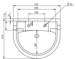
DIAGRAMS NOT TO SCALE | ALL DIMENSIONS IN MM TOLERANCE OF  $\pm$  5MM  ${\rm ALL\ PRODUCTS\ CONFORM\ TO\ BRITISH\ STANDARDS}$
