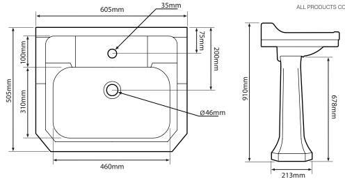
\*Dimensions are subject to change, customers are advised to measure actual product before commencing installation. \*\*Fixing point dimensions are for guidance only. The positions of fixings must be checked when product is received.
