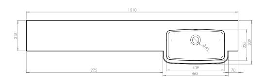
\*Right hand basin shown Mirror dimensions for left hand basin Diagrams not to scale All dimensions in mm Tolerance of +/-5mm
