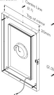
2.3 - Place the mirror body to one side. Drill the marked out positions and fit the wall plugs accordingly.
