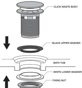
For the best flow rate from the overflow channel, ensure that the overflow slots in the waste and bath tub waste are fully aligned.
