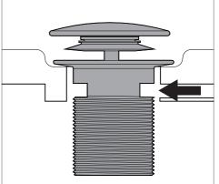
Please note: an overflow channel is to be used to prevent overflowing in an emergency and not to be relied upon when filling a bathtub.
