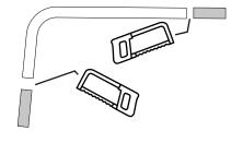
Measure the length of pipe required for the installation and cut down to length with a hacksaw or pipe cutter. Ensure sufficient length is kept to make a seal within the bath tub P trap.
