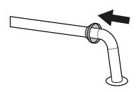
Before connecting the waste pipe to the waste or the bath tub, ensure the covering shroud is on the pipe with the large end facing towards the floor or wall.
