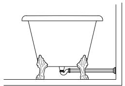
If the waste pipe runs out through the wall, then only the long end of the pipe is required and the short end and the bend of the pipe can be cut off.
