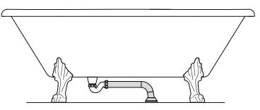
If the waste pipe runs out through the floor, then the long end of the pipe should be connected to the P Trap coming from the bath and the short end should be connected to the waste system.
