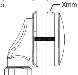
Measure the distance Xmm of excess fixing screw and remove X+5mm from the end of the screw using a hacksaw.
