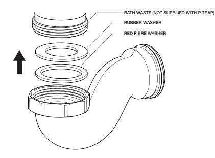
The P Trap can be connected to any waste fitting that has a 1 1/2" BSP screw fit connection.
