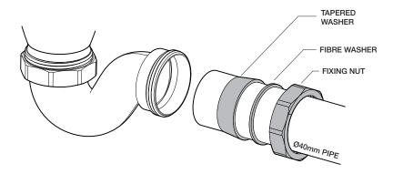
The P Trap can be connected to any 40mm waste pipe using the compression fitting. Place the black nylon into the locking nut and feed them over the 40mm pipe. Place the rubber washer over the 40mm pipe with the taper on the rubber washer facing into the P Trap so the narrow end is closer to the end of the pipe, as shown above.
