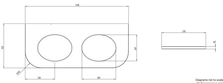
All dimensions in mm tolerance of +/-5mm
