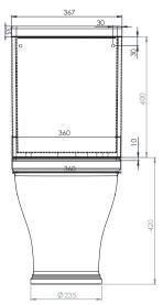
DIAGRAMS NOT TO SCALE | ALL DIMENSIONS IN MM | TOLERANCE OF  $\pm$  5MM  $\,$  ALL PROCUCTS CONFORM TO THE BRITISH FIXING STANDARDS
