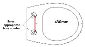
3 Once the 430mm dimension shown above is met and the template is parallel to the back edge, insert the bolts then tighten using a screw driver.
