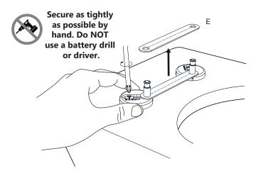
Remeasure the distance, making sure the 430mm dimension is met and remove the template and add the cover cap.
