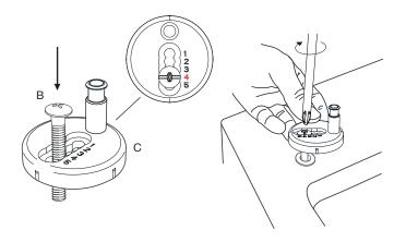
Using the anchor template provided, place over the two pins, making sure the template is parallel to the back of the pan and the pins are facing toward the bowl.
