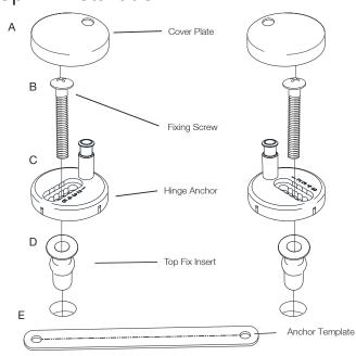
Note - alternative nuts and washers are supplied if you wish to secure the seat from underneath the deck of the toilet pan. If so dispose of the black top fix inserts and tighten with the securing key supplied.
