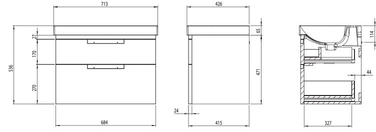
Diagrams not to scale All dimensions in mm tolerance of +/-5mm
