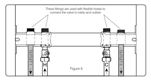
4. With the water inlet supplies installed, install outlet pipework using suitable plumbing fittings. Ensure that there is enough room to route pipework to the chosen outlet location.
