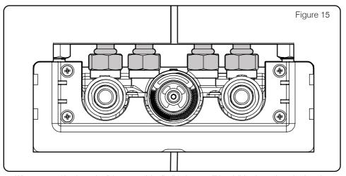
14. When secured in place, the fixing nuts of the flexible hoses will be visible above the valve housing. This will allow the connections to be checked for leaks and for the hoses to be tightened slightly, if necessary, without removing the entire valve.
