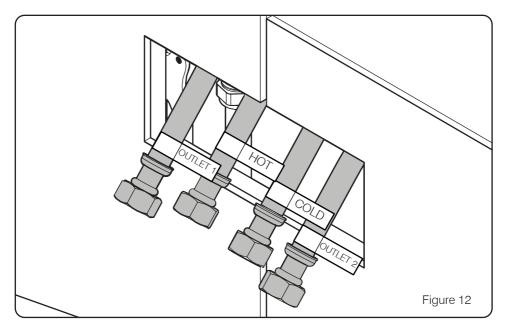
11. Pull the flexible hoses through the access hole in the wall and remove the zip tie.
