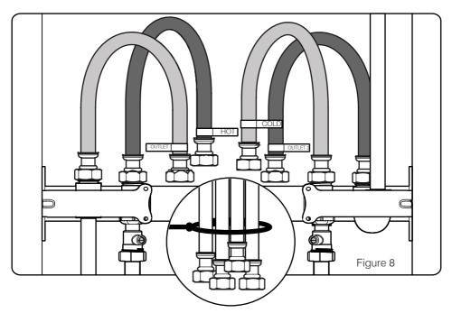
7. Once satisfied that there are no leaks, turn the water supply off and disconnect the valve from the flexible hoses. Before installing plasterboard and tiles, use the zip tie provided to tie the ends of the hoses together to make them easier to access later.
