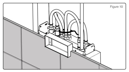
9. Once a hole has been cut in the plasterboard, secure it to the stud. The tile guide should pass through the hole in the plasterboard. Tile up to the edges of the tile guide to ensure the correct size access hole. Failure to do so may mean the cover plate does not form a water-tight seal in later installation stages.
