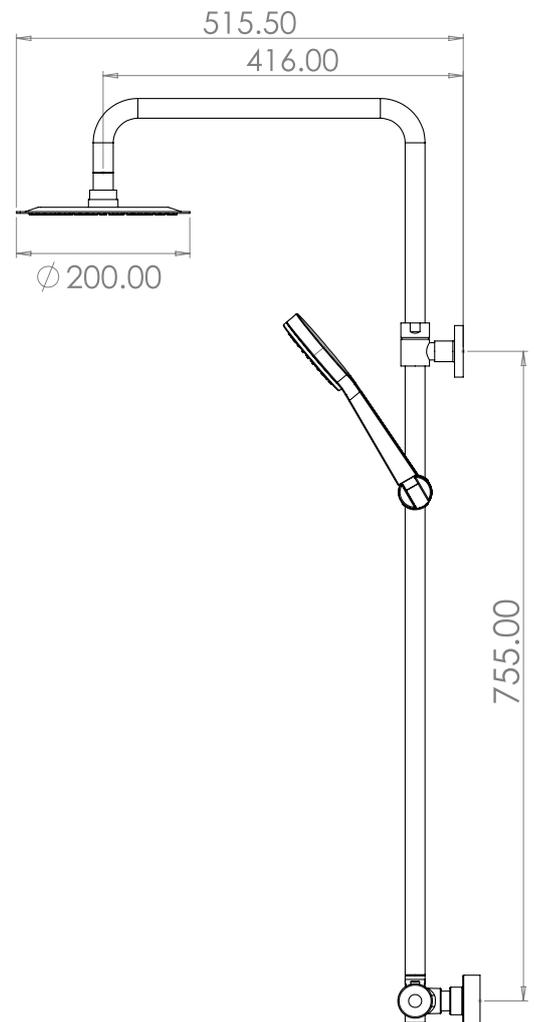
Riser rail adjustment - MIN 765mm MAX 1165mm.
