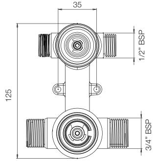
NOTE: VALVE TO BE RECESSED 80-100mm FROM FINISHED WALL SURFACE
