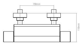
STORM BOTTOM OUTLET BAR VALVE SHOWN
