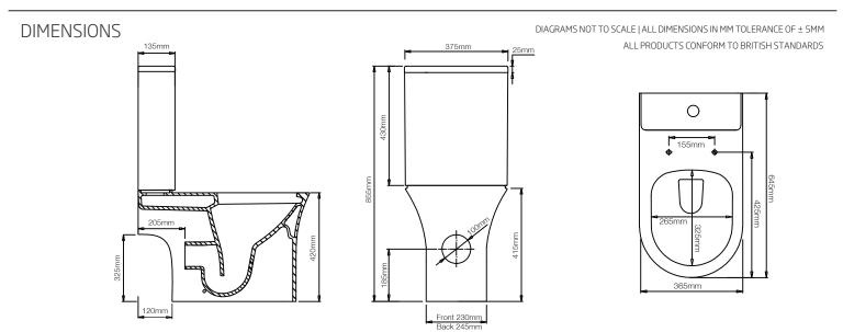
\*Dimensions are subject to change, customers are advised to measure actual product before commencing installation. \*\*Fixing point dimensions are for guidance only. The positions of fixings must be checked when product is received.
