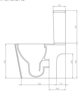
DIAGRAMS NOT TO SCALE | ALL DIMENSIONS IN MM TOLERANCE OF  $\pm$  5MM  ${\it ALL PRODUCTS CONFORM TO BRITISH STANDARDS} \\$
