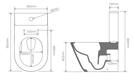
DIAGRAMS NOTTO SCALE | ALL DIMENSIONS IN MM TOLERANCE OF  $\pm$  5MM  ${\it ALL PRODUCTS CONFORM TO BRITISH STANDARDS }$
